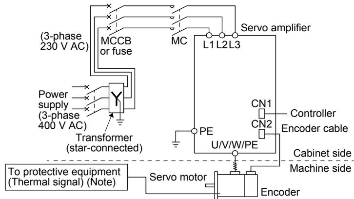
Note. Please use a thermal sensor, etc. for thermal protection of the servo motor.
