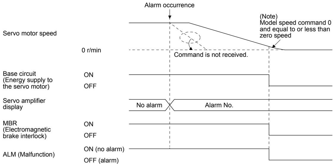
Note. The model speed command is a speed command generated in the servo amplifier for forced stop deceleration of the servo motor.
