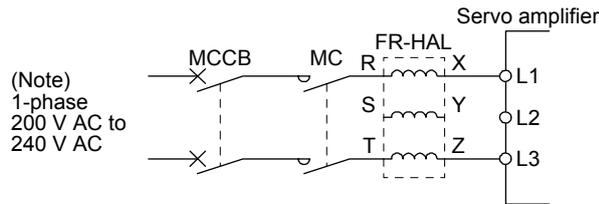
Note. Connect the power supply to L1 and L3. Leave L2 open.
