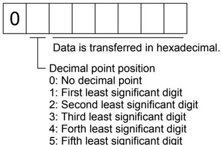
For example, here is described how to process the set data when a value of "15.5" is sent. Since the decimal point position is the second least significant digit, the decimal point position data is "2".
