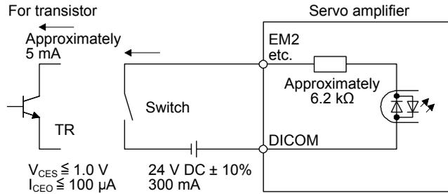
The following shows when the CN1-10 pin and the CN1-35 pin are used as digital input interface:
