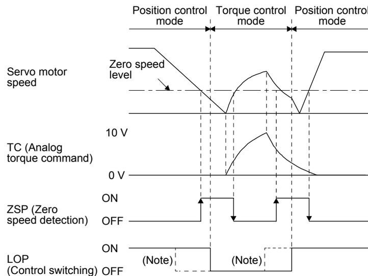
Note. When ZSP is not turned on, the control mode is not switched even if LOP is turned on/off. After LOP is turned on/off, even if ZSP is turned on, the control mode is not switched.
