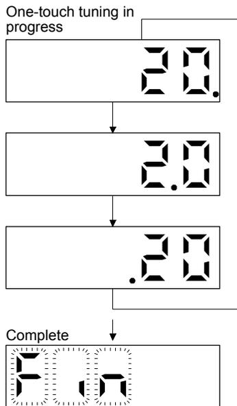
The one-touch tuning progress is displayed with 0% to 100%. The decimal point moves left to right in rotation during the tuning. To switch the display to the status display during the tuning, push the "MODE" button.
