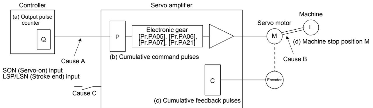
When a position shift occurs, check (a) output pulse counter Q, (b) cumulative command pulse P, (c) cumulative feedback pulse C, and (d) machine stop position M in the above diagram.
