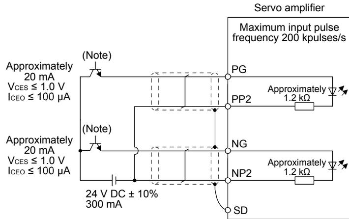
Note. Pulse train input interface is comprised of a photocopier.
