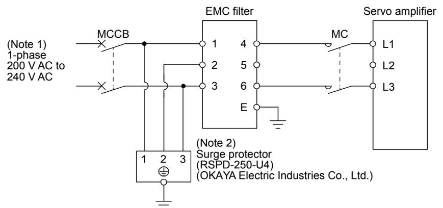
Note 1. Connect the power supply to L1 and L3. Leave L2 open.
