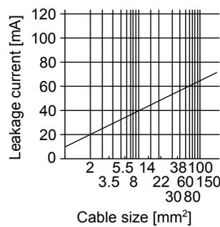
Fig. 11.2 Example of leakage current per km (I<sub>g1</sub>, I<sub>g2</sub>) for CV cable run in metal conduit
