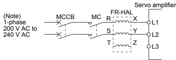
Note. Connect the power supply to L1 and L2. Leave L3 open.
