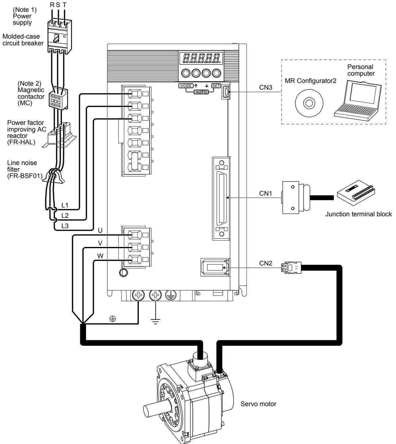
Note 1. For the power supply specifications, refer to section 1.3.
