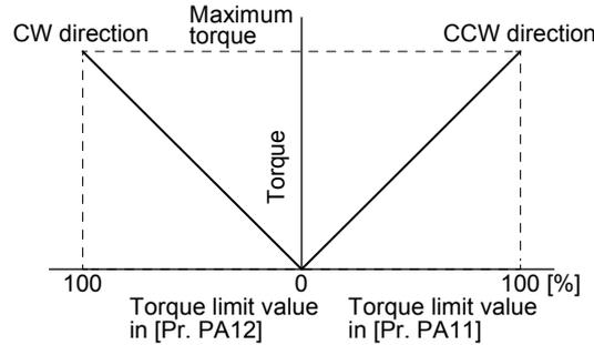
A relation between the applied voltage of TLA (Analog torque limit) and the torque limit value of the servo motor is as follows. Torque limit values will vary about 5% relative to the voltage depending on products. At the voltage of less than 0.05 V, torque may vary as it may not be limited sufficiently. Therefore, use this function at the voltage of 0.05 V or more.
