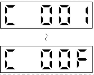
If an error occurs during the one-touch tuning, the tuning will be forcibly terminated and the stop symbol and error code from "C 001" to "C 00F" will be displayed by turns with 2 s interval.
