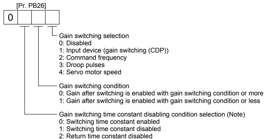
Note. This parameter setting is available with servo amplifiers with software version B4 or later.
