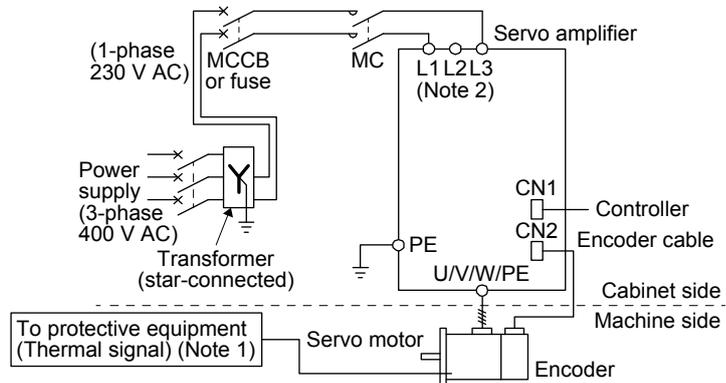
Note 1. Please use a thermal sensor, etc. for thermal protection of the servo motor.
