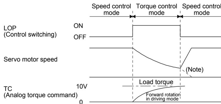
Note. When ST1 (Forward rotation start) and ST2 (Reverse rotation start) are switched off as soon as a mode is switched to the speed control, the servo motor comes to a stop according to the deceleration time constant. A shock may occur at switching control modes.
