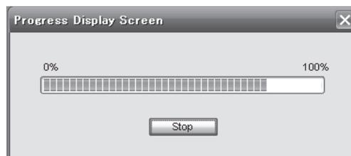
Completing the one-touch tuning starts writing tuning parameters to the servo amplifier. "0 0 0 0" is displayed at status in error code. In addition, settling time and overshoot amount will be displayed in "Adjustment result" after adjustment.
