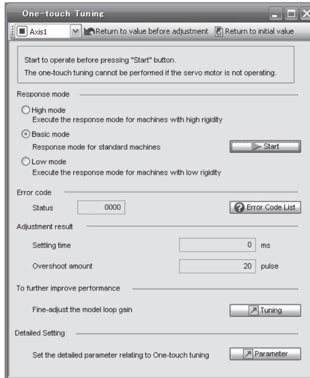
When clearing one-touch tuning is completed, the following window will be displayed. (returning to initial value)
