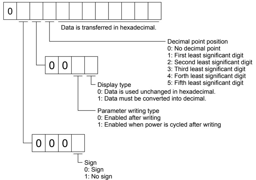
For example, data "00120000270F" means 999.9 (decimal display format) and data "000000003ABC" means 3ABC (hexadecimal display format).
