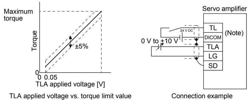
Note. This diagram shows sink I/O interface. For source I/O interface, refer to section 3.9.3.
