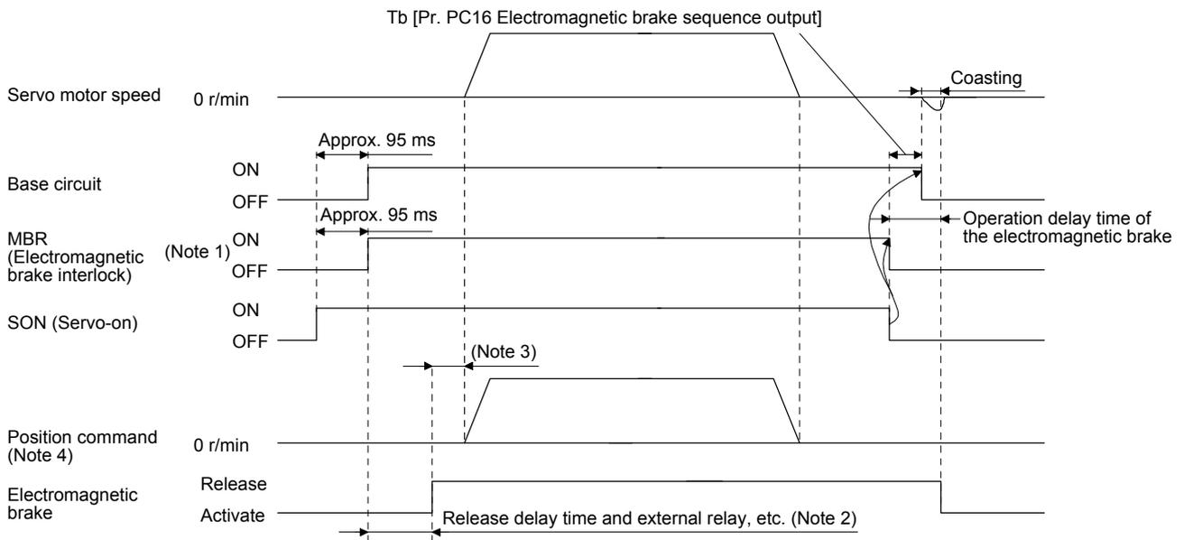
Note 1. ON: Electromagnetic brake is not activated.
