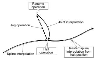
Fig.7-12:Behavior during halt and resume
