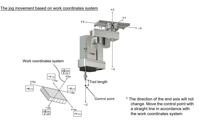
• When the[+X (J1)] keys are pressed, the robot will move along the X axis (Xw) plus direction on the work coordinates system.
