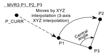
Fig.4-32:Example of circular interpolation motion path 3
