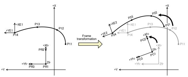
Fig.7-23:Frame transformation (Ex-T spline interpolation)
