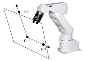
As can be seen in the diagram to the left, any plane can be defined by three points (P1, P2, and P3).
