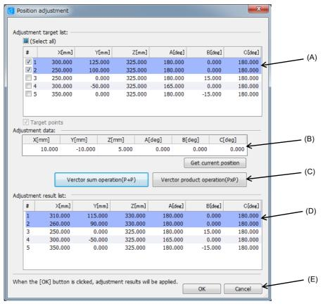
Fig.7-105:Position adjustment screen
