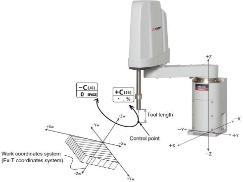
• When the [+C (J6)] keys are pressed, the control point will rotate in the plus direction around the Z axis (Zw) of work coordinates system (Ex-T coordinates system).
