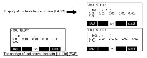
4) Press the function key assigned for "CLOSE" and finish.
