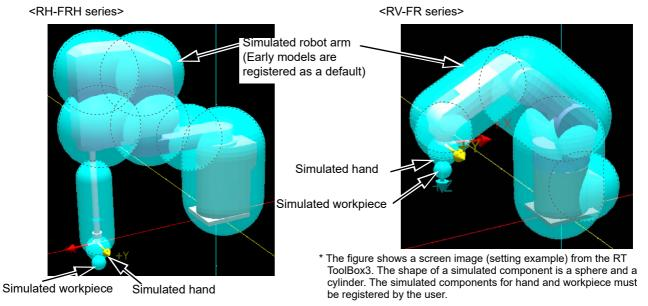
Fig.5-16:Example of simulated component registration
