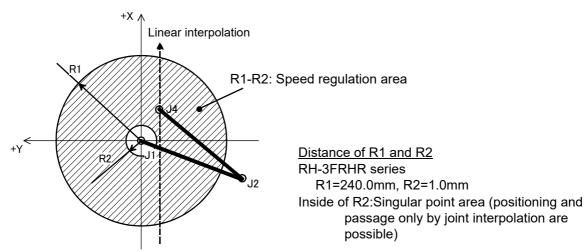
Fig.4-40:Speed regulation area and singular point area
