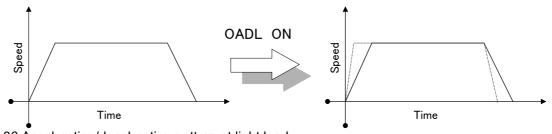
Fig.4-36:Acceleration/deceleration pattern at light load
