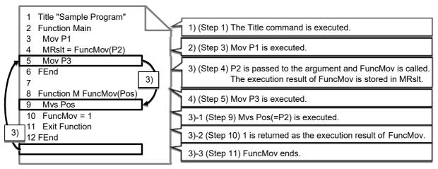
Fig.4-5:Flow of processing with the Function procedure
