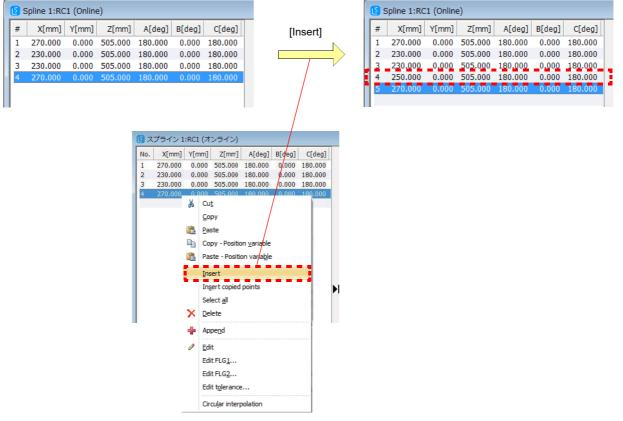
Fig.7-53:Inserting path point data
