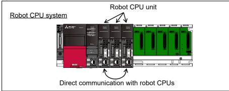
Fig.5-26:Direct communication with robot CPUs
