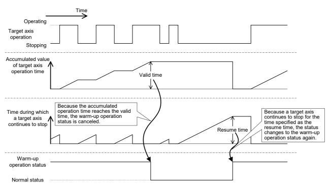
Fig.5-5:Example of Switching Between the Normal Status and the Warm-Up Operation Status
