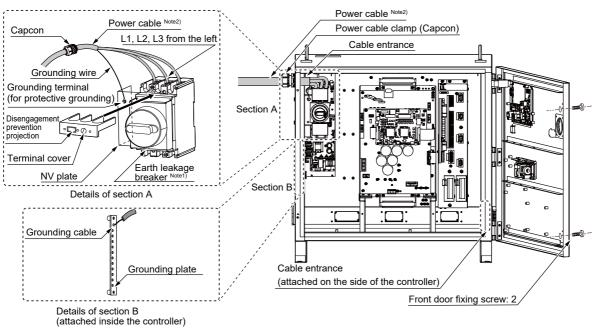
Note 1) Always use the terminal cover for the earth leakage breaker.
