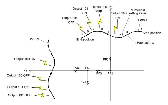
Fig.7-103:Movement of sample program
