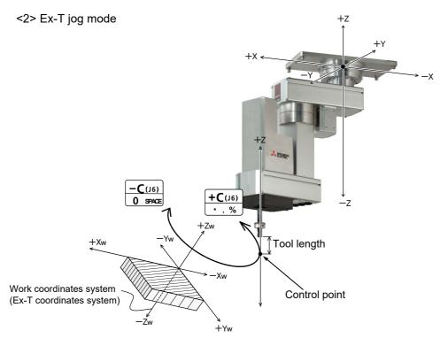
• When the[+C (J6)] keys are pressed, the Z axis will rotate in the plus direction of the XYZ coordinate system.
