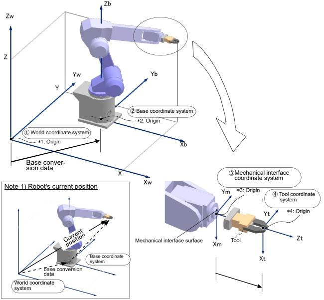
Fig.4-7:Robot's coordinate system
