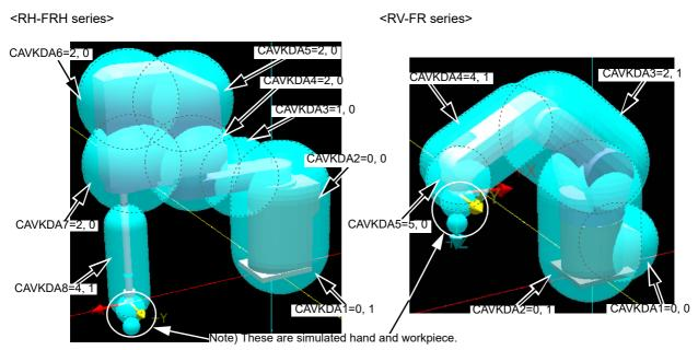
Fig.5-19:Example of registration sections and simulated component type settings
