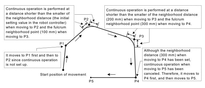
Fig.4-20:Example of continuous path operation
