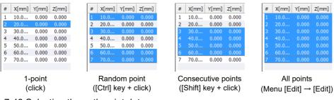
Fig.7-48:Selecting the path point data
