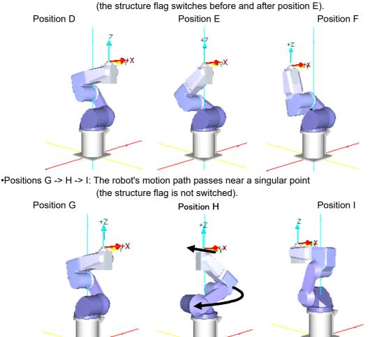
CAUTION When passing near a singular point, the robot may rotate in a wide circle as in the case of position H in the figure above. Be sure to keep an eye on the robot and avoid getting in the way when working near the robot, such as when teaching positions.
