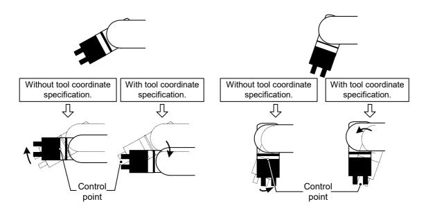
If tool coordinates are specified with the TOOL command or parameters, the hand will be aligned at the specified tool coordinates. If not specified, the hand will be aligned at the center of the mechanical interface. The illustration above shows an example of a vertically articulated robot. "With Tool Coordinate Specification" indicates when the tool coordinates are specified at the tip of the hand. For further information on tool coordinates, refer to Page 529, "5.6 Standard Tool Coordinates".
