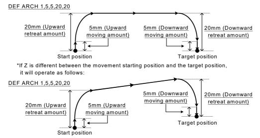
Fig.4-26:Example of arch interpolation motion path (seen from the side)
