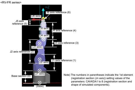
Fig.5-18:Registration sections of simulated components of RV-FR series (supplement)
