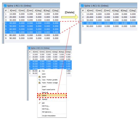
Fig.7-55:Deleting the path point data
