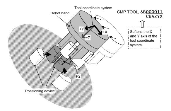
Fig.4-19:The example of using the compliance mode
