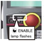
The status display lamp "ENABLE" on the front of the T/B blinks.
