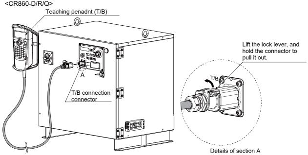
Fig.2-2:Installing and removing the T/B
