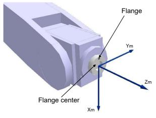
Fig.4-10:Mechanical interface coordinate system
