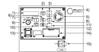
Fig.2-3:Part names of the operation panel (CR860 controller)
