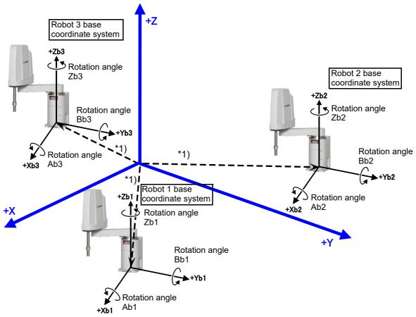
\*1) The robot's base coordinate system origin point looking from the common coordinate system. Set these coordinate values in parameter: RBCORD for each robot.
