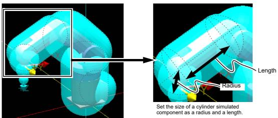
Fig.5-21:Simulated component size (supplement)
