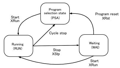
Fig.4-2:Operation state of each slot
