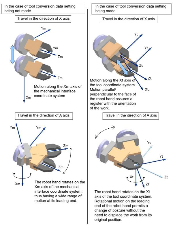
Fig.4-13:Tool jogging operation with/without tool conversion data
