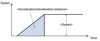
Fig.4-35: Acceleration with <Acceleration/deceleration distance>
