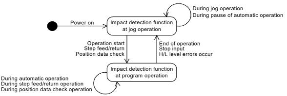
Fig.5-8:State transition diagram illustrating switch between program operation and jog operation
