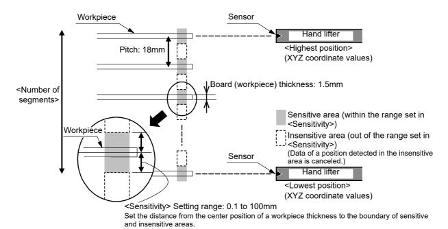
Fig.4-23: Sensitive area of a sensor
