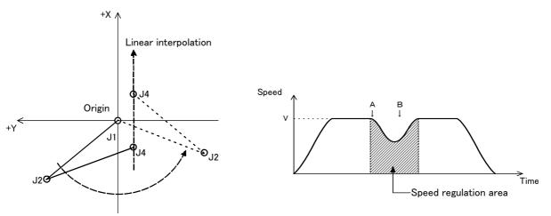
Fig.4-38:Passing through near the origin point
