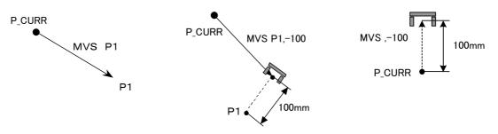
Fig.4-33:Example of movement at linear interpolation
