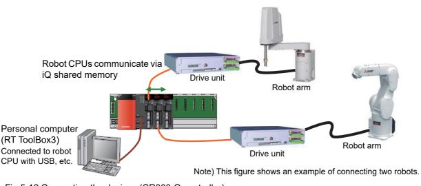
Fig.5-12:Connecting the devices (CR800-Q controller)
