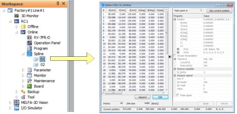
Fig.7-44:Opening a spline file saved in the controller
