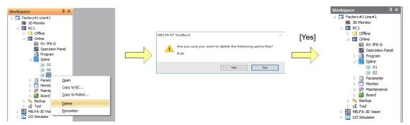
Fig.7-66:Deleting a spline file
