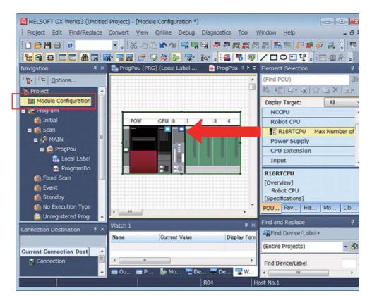
Fig.6-1:GX Works3 module configuration screen (one robot)
