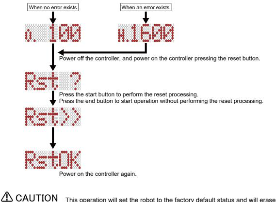
This operation will set the robot to the factory default status and will erase parameters, programs, and various log data. Do not perform this operation unless an error (H1600) has occurred. The erased data can be restored using the restore function if batch backup data has been saved in RT ToolBox3 (option).
