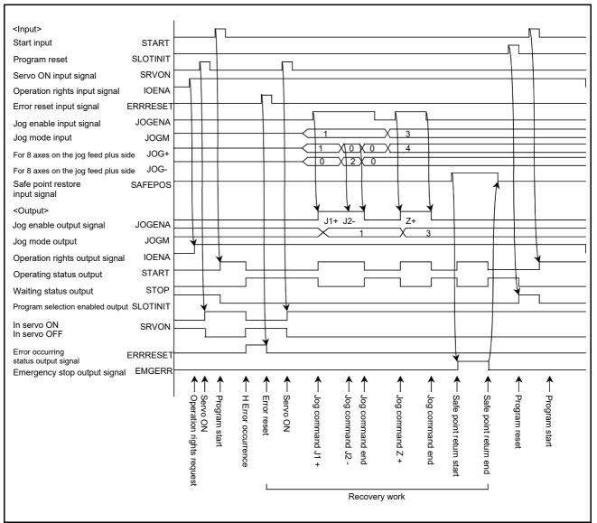
Fig.6-8:Example of external operation timing chart (Part 4)
