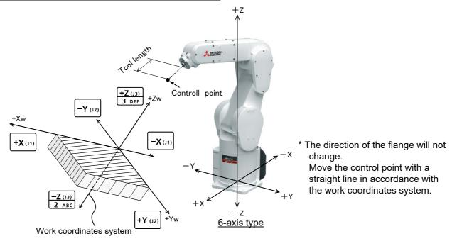
• When the[+X (J1)] keys are pressed, the robot will move along the X axis (Xw) plus direction on the work coordinates system.
