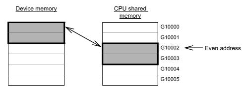
Fig.4-42:Preventing data inconsistency of 32-bit data
