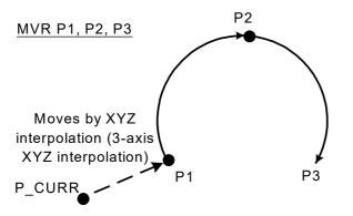
Fig.4-30:Example of circular interpolation motion path 1
