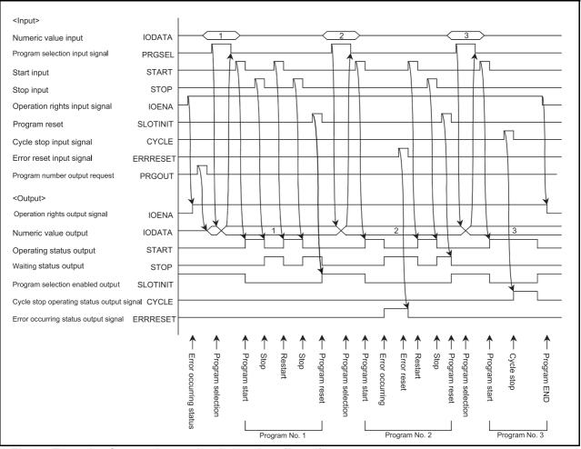
Fig.6-5:Example of external operation timing chart (Part 1)
