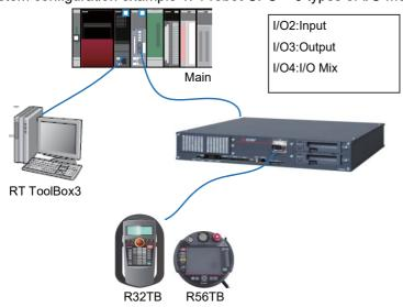
\*System configuration example 2: 2 robot CPUs + 3 types of I/O modules + extension base (added)
