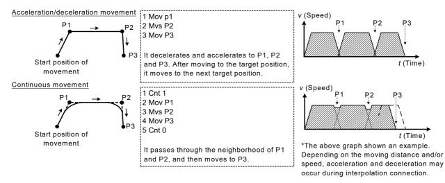
Fig.4-21:Acceleration/deceleration movement and continuous movement
