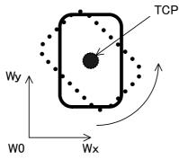
Fig.7-117:Example of C element movement in the WORK jog
