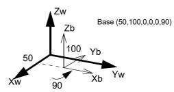
Fig.4-16:Conceptual diagram of the base coordinate system
