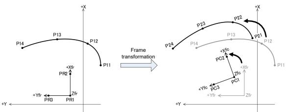
Fig.4-37: Example of frame transformation
