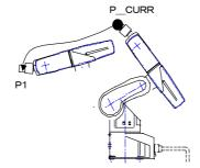
Fig.4-25:Example of joint interpolation motion path
