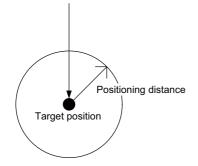
"Positioning is completed when the current position moves into the sphere with the radius specified in <Positioning Distance>."
