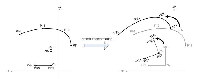
Fig.7-22:Frame transformation (Spline interpolation)
