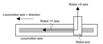
In this case, parameter AXDIR is set to 0.0, 0.0, -90.0. (-90 degree rotation around robot's Z axis.)
