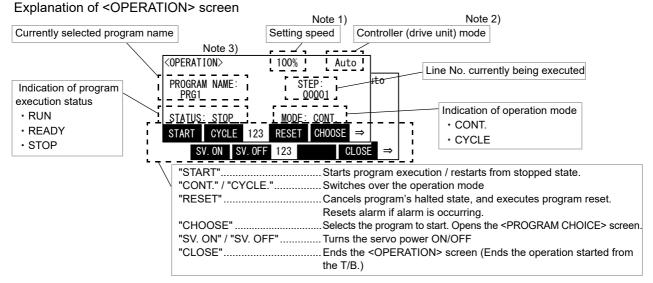
Note 1) When the controller mode is "MANUAL", the robot moves at low speed even if the set speed is 100%. (For operation check) Note 2) When the controller mode is "AUTOMATIC", the T/B's status display lamp [ENABLE] blinks to indicate that the T/B is enabled. The T/B is disabled when the <OPERATION> screen is ended.
