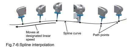
• A file dedicated for spline interpolation (spline file) in which the path point data is registered is used separately from the robot program. This file is created and edited in the RT ToolBox3 dedicated edit screen (Spline File Edit screen), and written to the controller.
