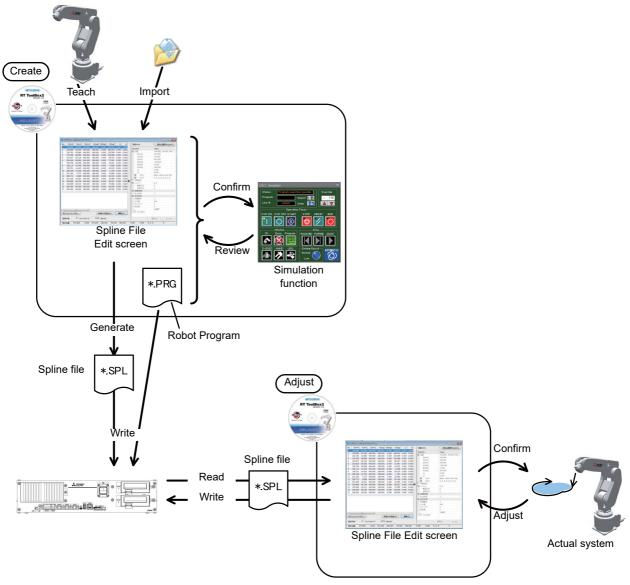
Fig.7-24:Schematic diagram of work details
