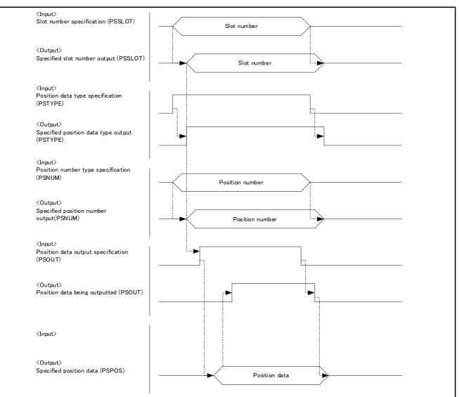
Fig.6-9:Example of external operation timing chart (Part 5)
