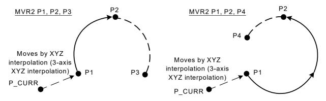
Fig.4-31:Example of circular interpolation motion path 2
