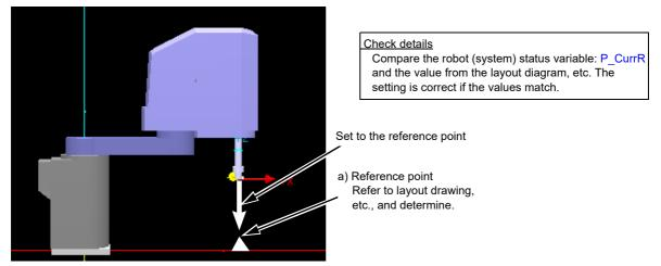
Fig.5-25:Checking the setting for calibration between robots
