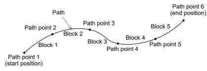
Fig.7-9:Spline interpolation terminology
