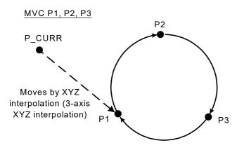
Fig.4-29:Example of circle interpolation motion path
