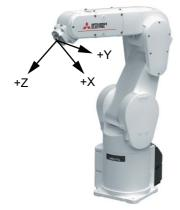
Definitions of Coordinate Axes The tool coordinate is used for the coordinate axes. Axes that must be set: The X, Y and Z elements of the center of gravity and the X, Y and Z elements of the size must be set.
