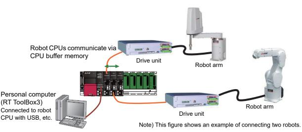
Fig.5-11:Connecting the devices (CR800-R controller)
