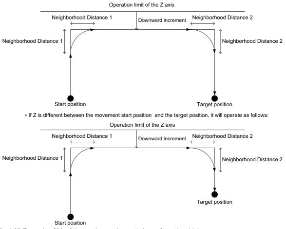
Fig.4-27:Example of Mva2 instruction motion path (seen from the side)
