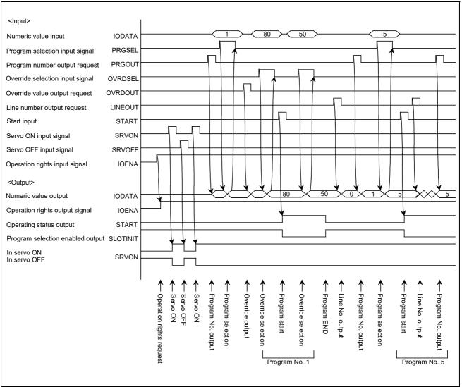
Fig.6-6:Example of external operation timing chart (Part 2)
