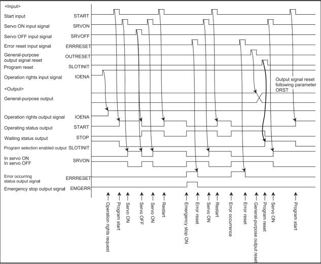
Fig.6-7:Example of external operation timing chart (Part 3)
