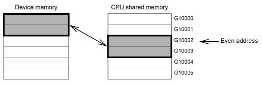
Fig.4-41:Preventing 32-bit data separation
