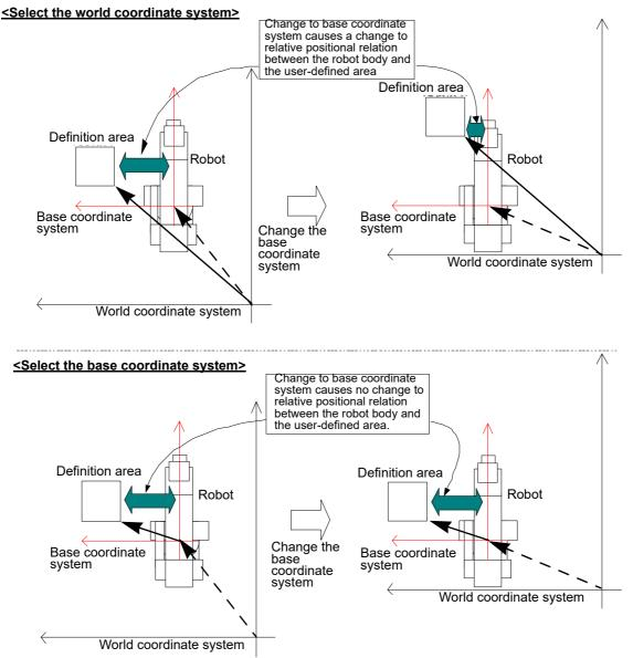
Note) A top-down view of a vertically articulated 6-axis robot is used as an example in these figures. The example also applies to horizontally articulated robots.
