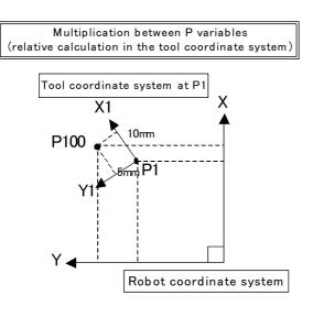
An example of relative calculation (multiplication) 1 P2=(10,5,0,0,0,0)(0,0) 2 <u>P100=P1\*P2</u> 3 Mov P1 4 Mvs P100
