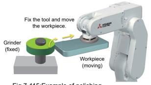
Fig.7-115:Example of polishing
