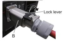
When removing the connector for T/B connection, use lock release (state which raised the lock lever to the up side), make the case of the B section slide to the front, and remove and pull up out the latch.
