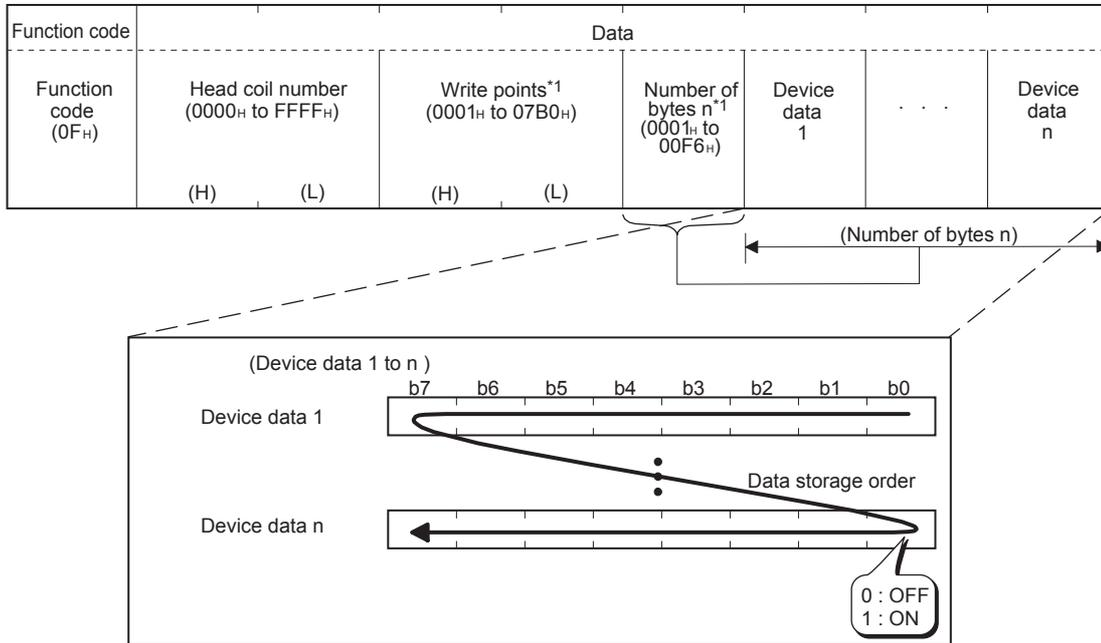
The values (ON/OFF) stored into the device data 1 to n are written to the coils in order from low-order to high-order bits of the device data.
