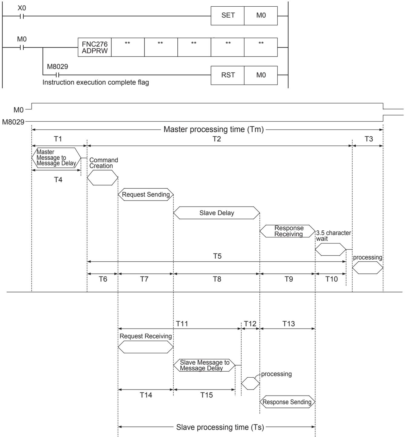
The Master processing time (T<sub>m</sub>) can be calculated in milliseconds (ms) as follows, where INT (n) indicates the concatenation of any remaining decimal values.
