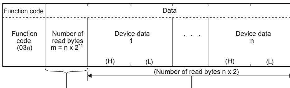
\*1 For example, if  $n = 4$ , the number of bytes is calculated as  $4 \times 2 = 8$  bytes
