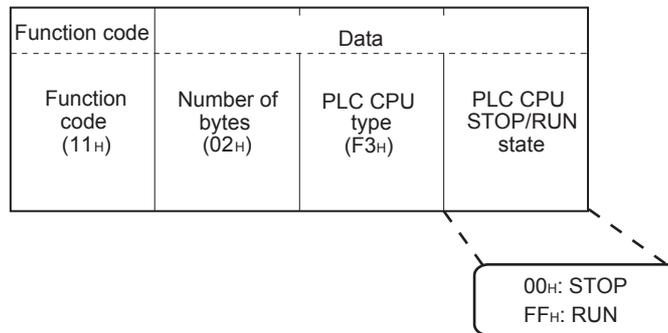
The slave (FX-Series MODBUS Communication ADP) will return 'F3' as the PLC CPU type data to the Master:
