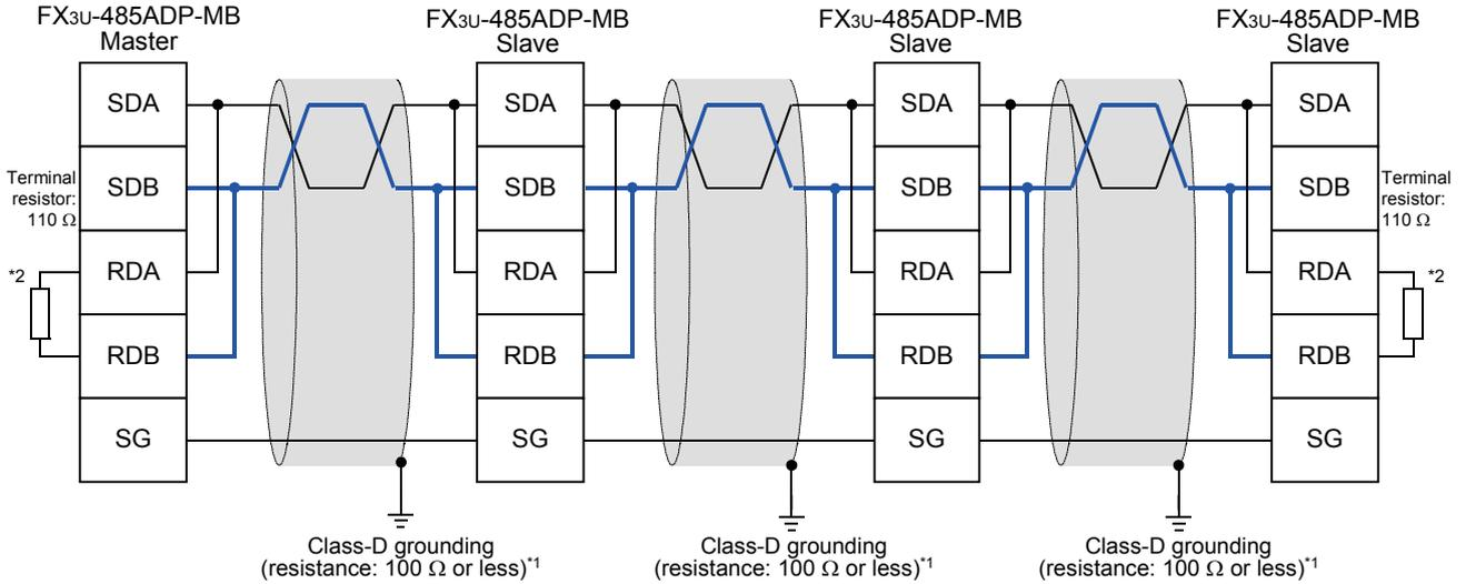
\*1 Make sure to perform Class-D grounding on the shield of the twisted pair cable connected to the FX3U-485ADP-MB.
