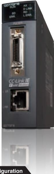
The CC-Link IE Field Network Simple Motion module is an intelligent function module performing positioning/synchronous/cam control with simple parameter settings, starting from the sequence program. QD77GF16 can be used as the master station of CC-Link IE Field Network.
